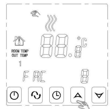
7. Press the power key, then the thermostat will be shutdown
